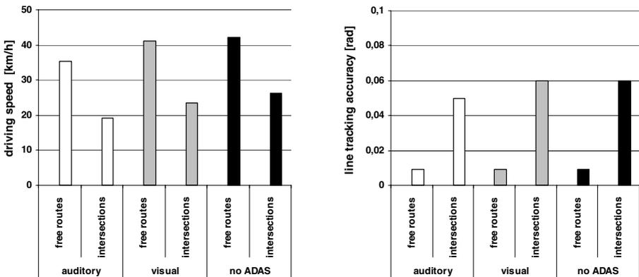
**Fig. 3.** Effects of ADAS modality on driving speed (left) and accuracy (right)
