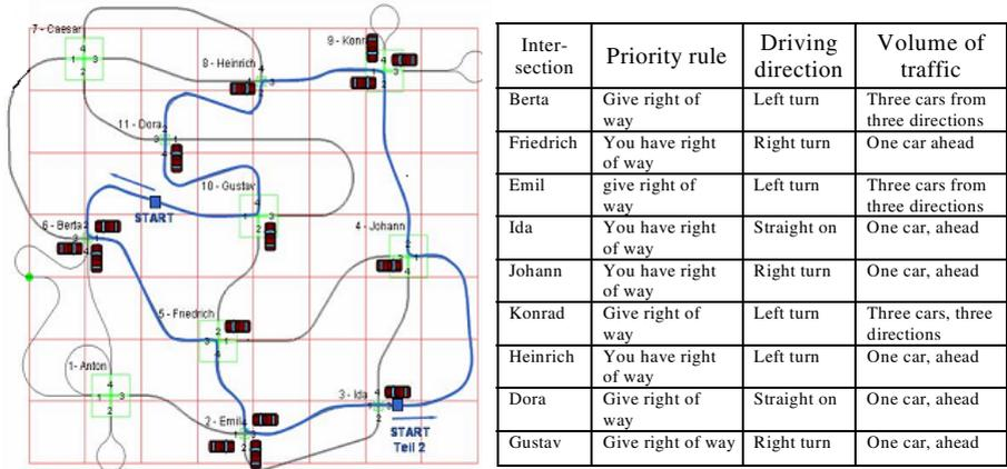
**Fig. 2.** Left side: Experimental route with nine different intersections; Right side: Priority rule, driving directions and volume of traffic at the different intersections
