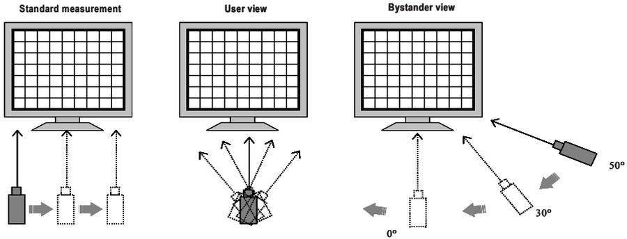
**Fig. 41.2:** Quantifying anisotropy: Left: “standard view”- the photometer is displaced at right angles; center: “user view”- the photometer emulates users’ head movements; right: “bystander view”- the photometer is positioned off-axis (ZIEFLE et al. 2003)
