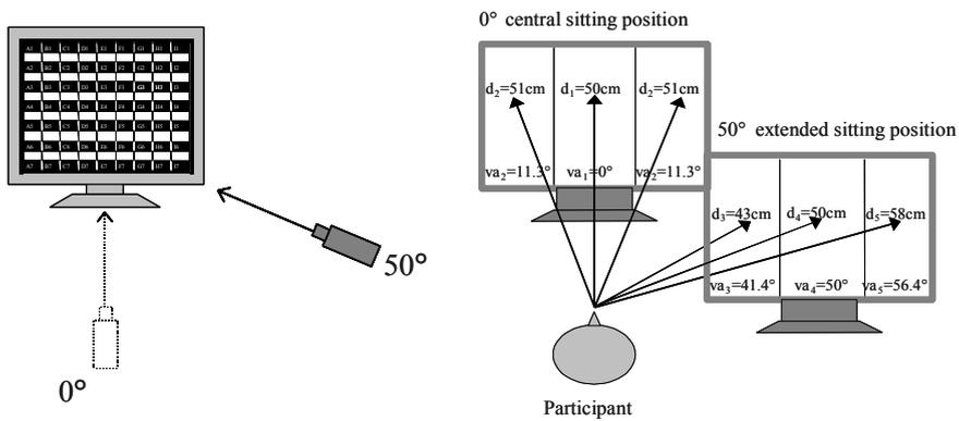
**Fig. 41.4:** Left: The photometer set up with the screen divided into 63 single fields; right: The experimental setting with the two sitting positions. By dividing the screen into three sections, five viewing angles can be distinguished (OETJEN & ZIEFLE 2007)
