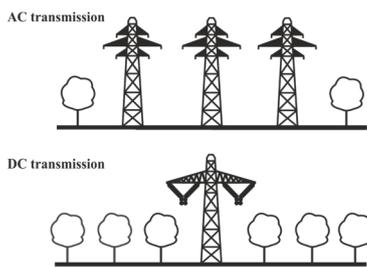
Figure 2: Space requirement of AC and DC overhead lines (“ABB review Special Report: 60 years of HVDC,” 2014).
