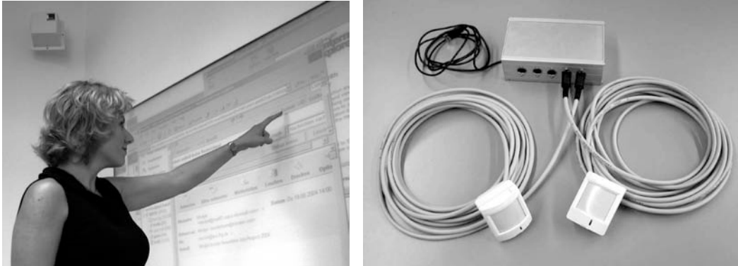
Figure 3: Large public display with an RFID antenna in upper left corner (left) and infrared detection system with two sensors (right).
