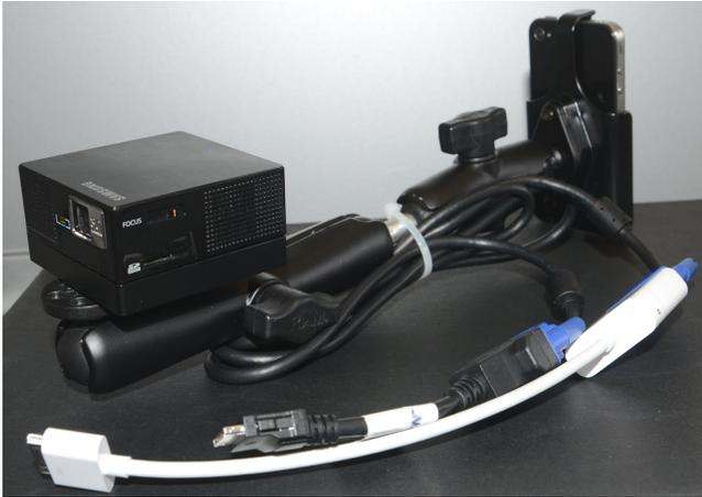
**Figure 2: The projector based navigator prototype (Dimension: 32x11.5x7 (cm) Weight: about 1kg)**
