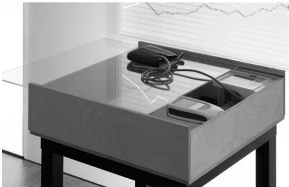
**FIGURE 4.** Device integration: blood pressure and coagulation monitoring device implemented in a table.
