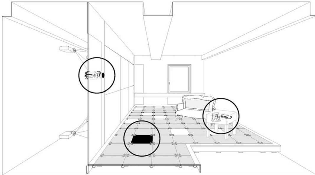
**FIGURE 3.** Visualization of the monitoring system in the Future Care Lab. From left to right: an infrared camera is integrated in the wall next to the display, weight sensors are installed under the entire floor (additionally a scale is installed under one floor tile in front of the display wall), and blood pressure and coagulation monitoring devices are implemented in a table.
