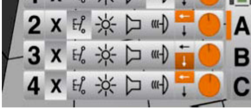
Fig. 3. Sensor configuration panel. Sensor 1 is configured as ultra-sound sensor sideways. Sensor 2 is configured as a touch sensor pointing ahead. Sensors 3 and 4 are disabled.
